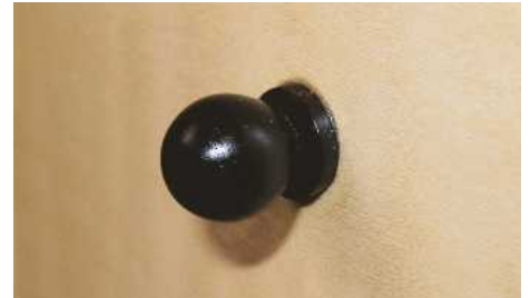
▲ Pic 21 The drawer pulls are turned in ebony with a 10mm diameter and 12mm collar
